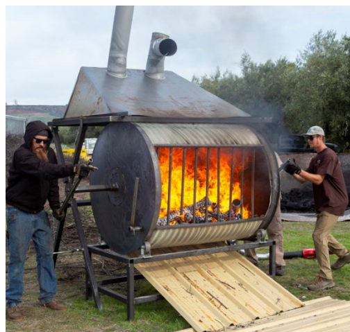
Figure 2. 4-ft diameter RoCC kiln, rear view, preparing to unload biochar. February 2020
