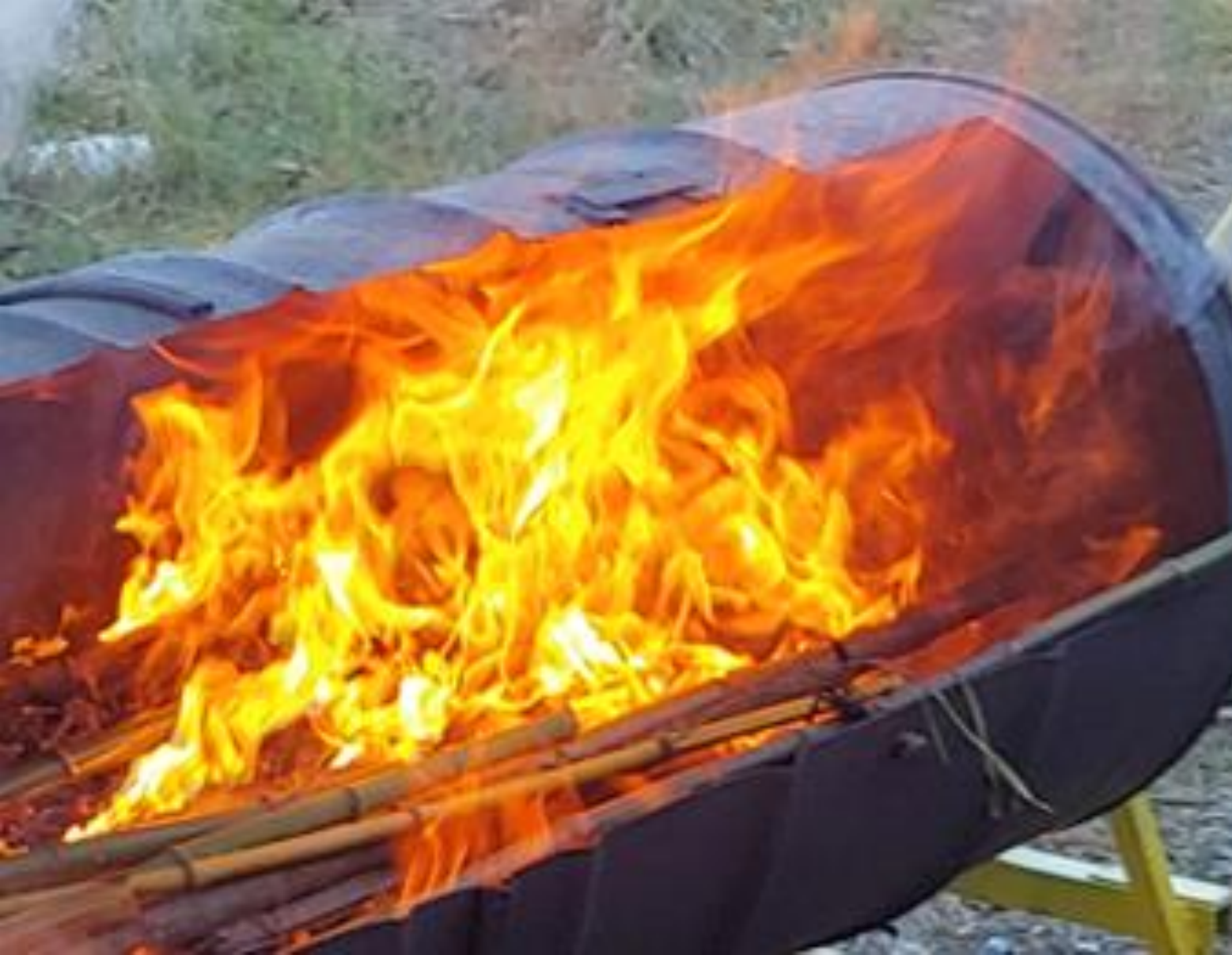
RoCC kiln: 2-barrel; Bamboo biochar small demonstration; 2023-12-05 North Carolina, USA.
